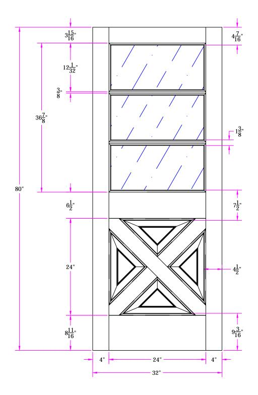
THIS DRAWING AND THE INFORMATION CONTAINED HEREIN IS PROPRIETARY TO TITLE 7335 2/8 x 6/8 SIMPSON DOOR COMPANY AND SHALL NOT BE REPRODUCED, COPIED OR DISCLOSED IN **Customer Layout** WHOLE OR PART, OR USED FOR MANUFACTURE OR FOR ANY OTHER PURPOSE WITHOUT THE WRITTEN PERMISSION OF SIMPSON DOOR COMPANY. DRAWING NO. D-7335-208-608-0700 Revisions SCALE NTS PATTERN # 7008 Rev. # Description Date by Whom DATE 10/29/2015 DRAWN J. Phinney **Simpson®**
