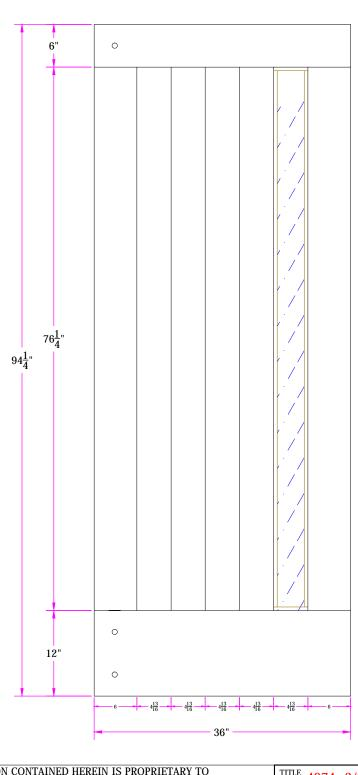
THIS DRAWING AND THE INFORMATION CONTAINED HEREIN IS PROPRIETARY TO TITLE 4974 3/0 x 7/10.25 SIMPSON DOOR COMPANY AND SHALL NOT BE REPRODUCED, COPIED OR DISCLOSED IN **Customer Layout** WHOLE OR PART, OR USED FOR MANUFACTURE OR FOR ANY OTHER PURPOSE WITHOUT THE WRITTEN PERMISSION OF SIMPSON DOOR COMPANY. DRAWING NO. D-4974-300-710.25-0800 Revisions SCALE NTS LAYOUT 000 PATTERN # 00000 Rev. # Description Date by Whom DRAWN J. Decker
