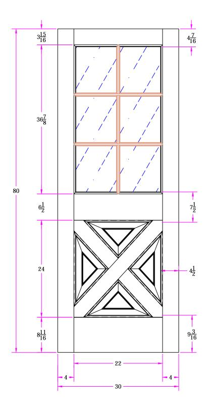
THIS DRAWING AND THE INFORMATION CONTAINED HEREIN IS PROPRIETARY TO TITLE 37635 2/6 x 6/8 SIMPSON DOOR COMPANY AND SHALL NOT BE REPRODUCED, COPIED OR DISCLOSED IN **Customer Layout** WHOLE OR PART, OR USED FOR MANUFACTURE OR FOR ANY OTHER PURPOSE WITHOUT THE WRITTEN PERMISSION OF SIMPSON DOOR COMPANY. DRAWING NO. D-37635-206-608-0700 Revisions SCALE NTS PATTERN # 7008 Rev. # Description Date by Whom DATE 10/29/2015 DRAWN J. Phinney **Simpson®**
