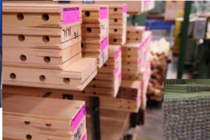
Bored to accept dowel pins
