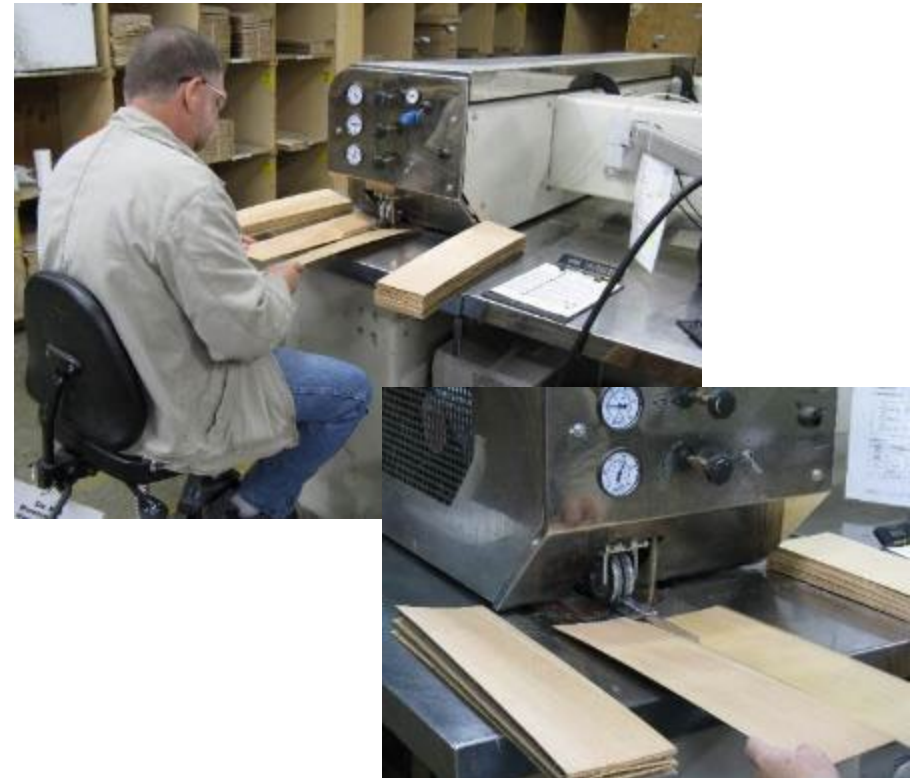
Stitching veneers together for wider components
