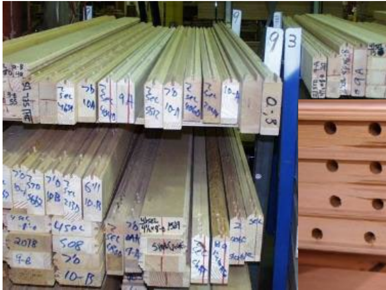
Components trimmed and profiled
