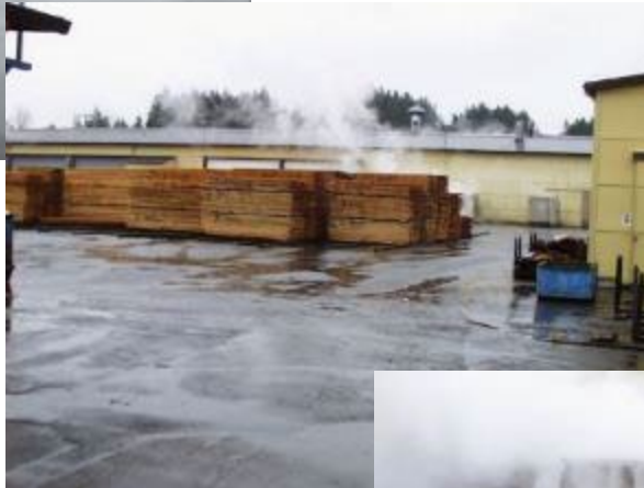
Sorted lumber - pre-conditioning prior to slicing veneers. Lumber ready to go to the kilns. 10-14 days in the kiln - slow controlled drying.
