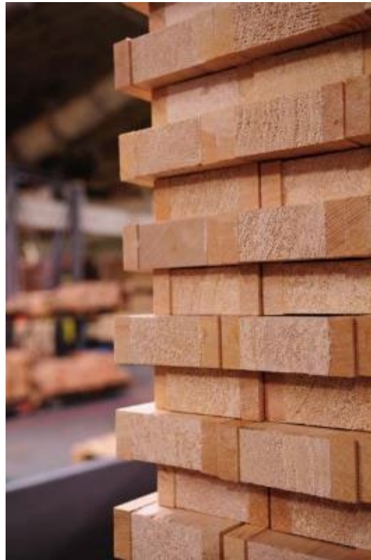
Core material with edge strips
