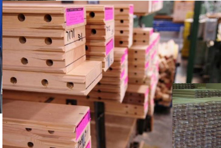
Bored to accept dowel pins
