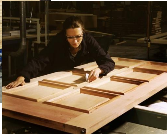
Final door inspection
