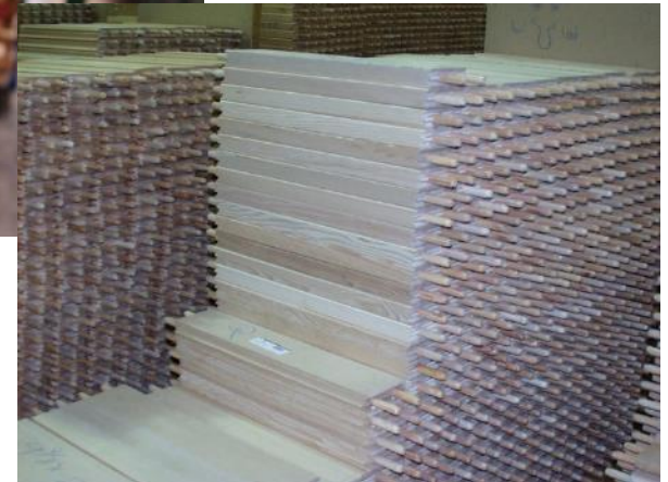
Rails with dowel pins inserted
