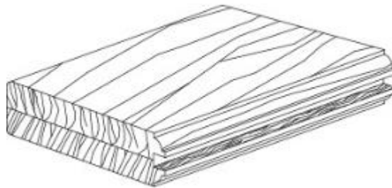
Solid 2-Piece Laminated Construction
