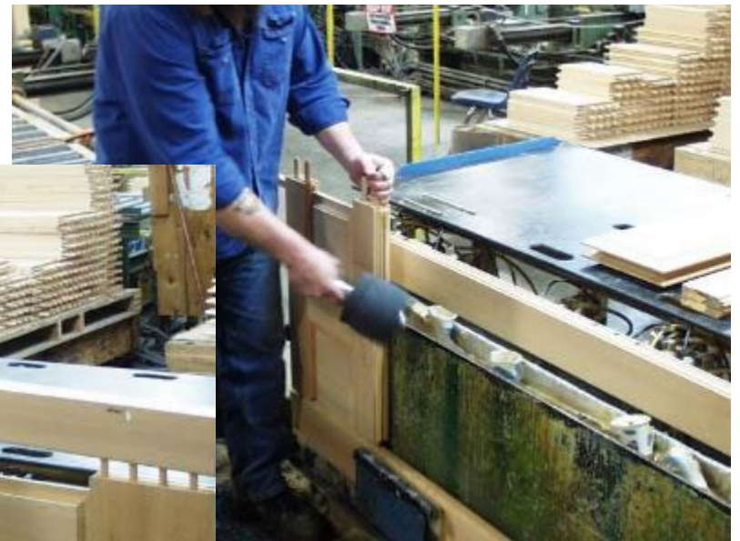
Assembled by hand by a door sapper
