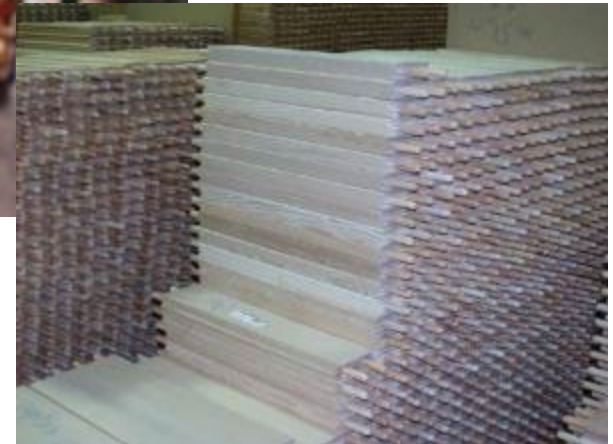
Rails with dowel pins inserted
