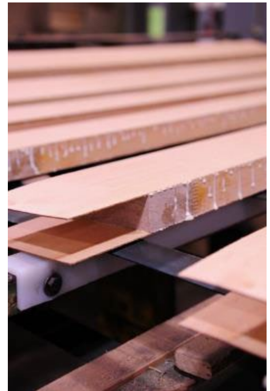
Veneers applied to face of component
